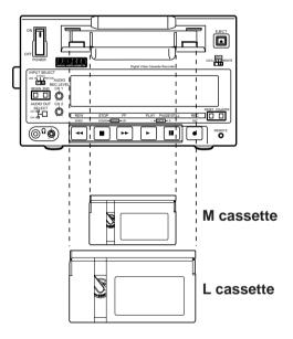
Align the cassette with the center of the insertion slot, and push it in gently.
